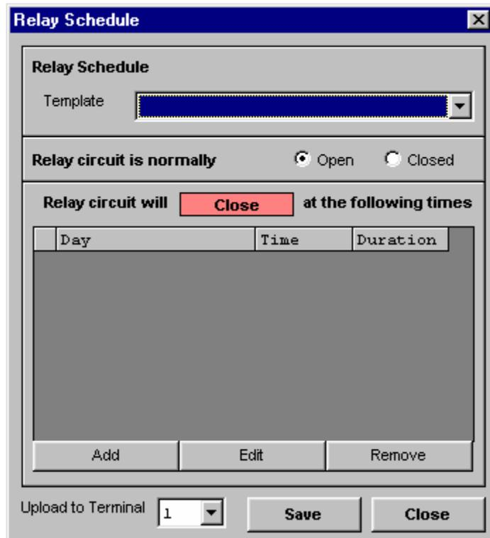
The screenshot shows a larger dialog box titled "Relay Schedule". It includes a "Template" dropdown menu, radio buttons for "Relay circuit is normally" (Open/Closed), and a section for "Relay circuit will" with a red "Close" button and the text "at the following times". Below this is a table with columns for "Day", "Time", and "Duration". At the bottom, there are "Add", "Edit", and "Remove" buttons, an "Upload to Terminal" dropdown (set to 1), and "Save" and "Close" buttons.
