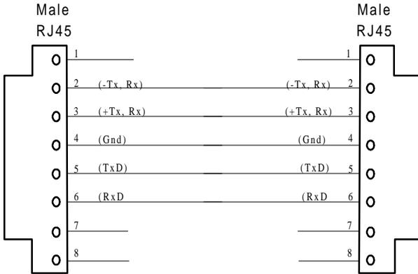
The RJ45 connector on the terminal side must be a short (12.35mm) RJ45 connector in order to enable the SY-780 connector case that hides the connectors to close.
